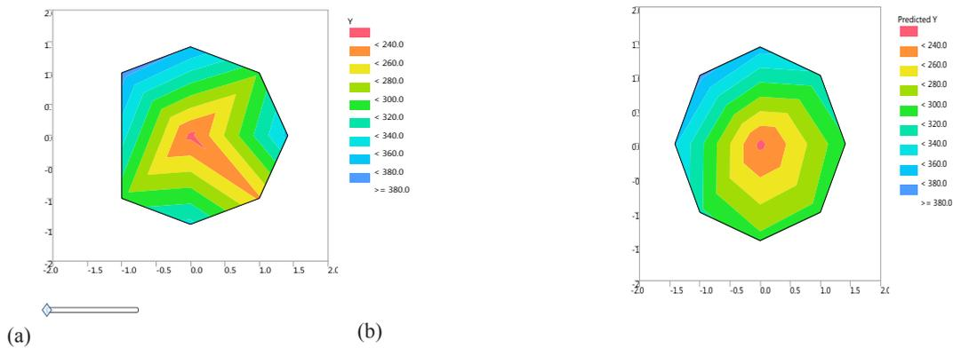
**Fig. 9. (a) Contour Plot for response Y (compressive strength) actual values, and (b) predicted values.**
