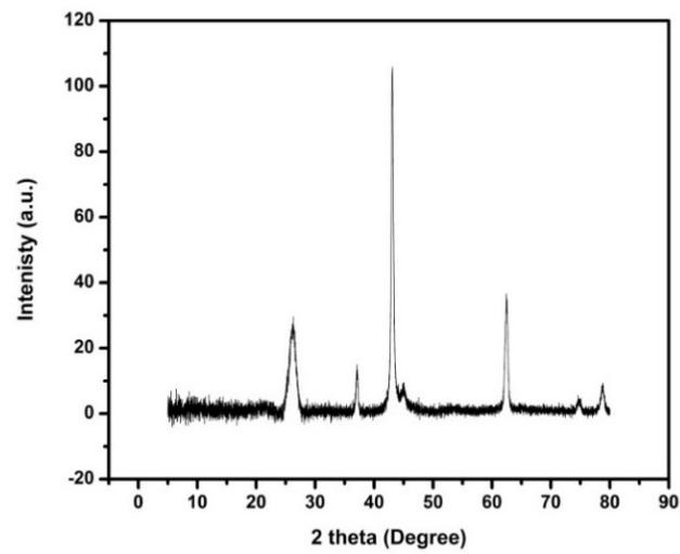
Fig. 2. XRD diffraction pattern of CNTs.
