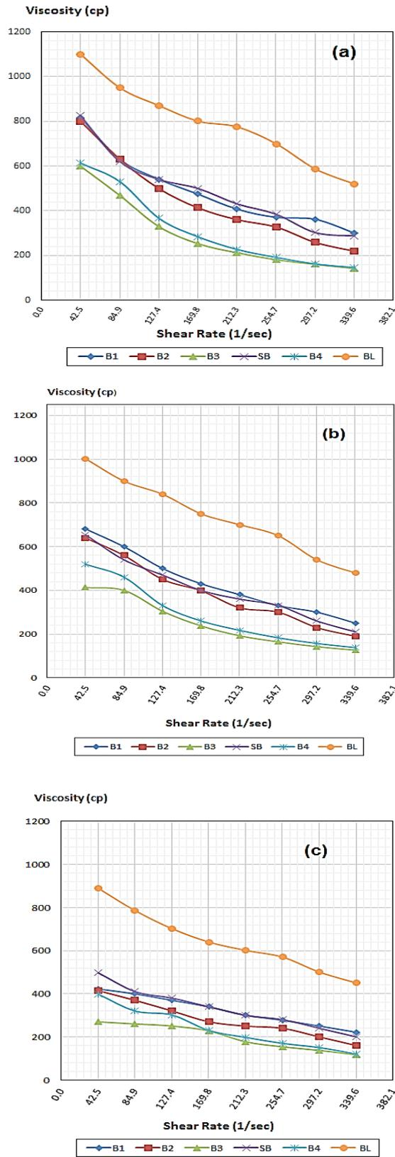
Fig. 6. Relation Between Shear Rate (1/sec) and Viscosity (Cp) for Treated and Untreated Crude Oil at Concentration 1000 ppm at Temperature a) 15 °C, b) 20°C, c) 30°C
