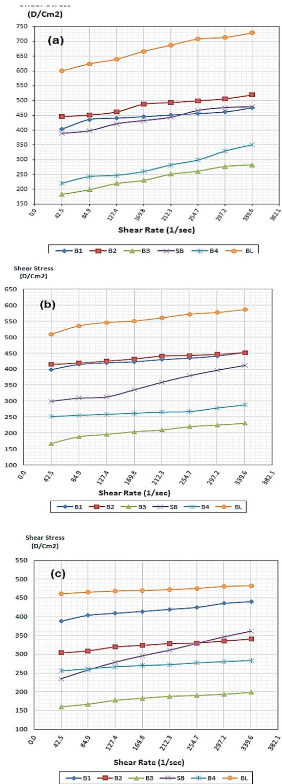
Fig. 5. Relation Between Shear Rate (1/sec) and Shear Stress (D/ Cm2) for Treated and Untreated Crude Oil at Concentration 1000 ppm at Temperature a) 15°C, b) 20°C, c) 30°C
