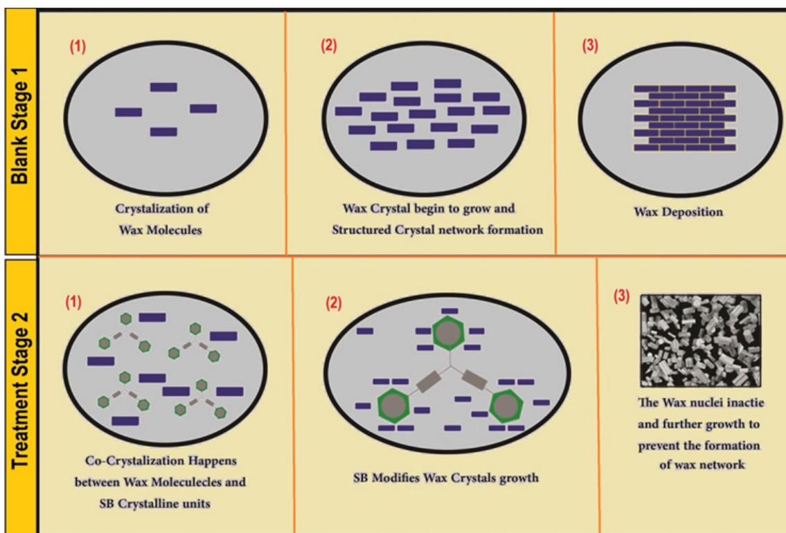
Fig. 7. Mechanism of Dispersion of Paraffin Wax Crude Oil by [SB1]
