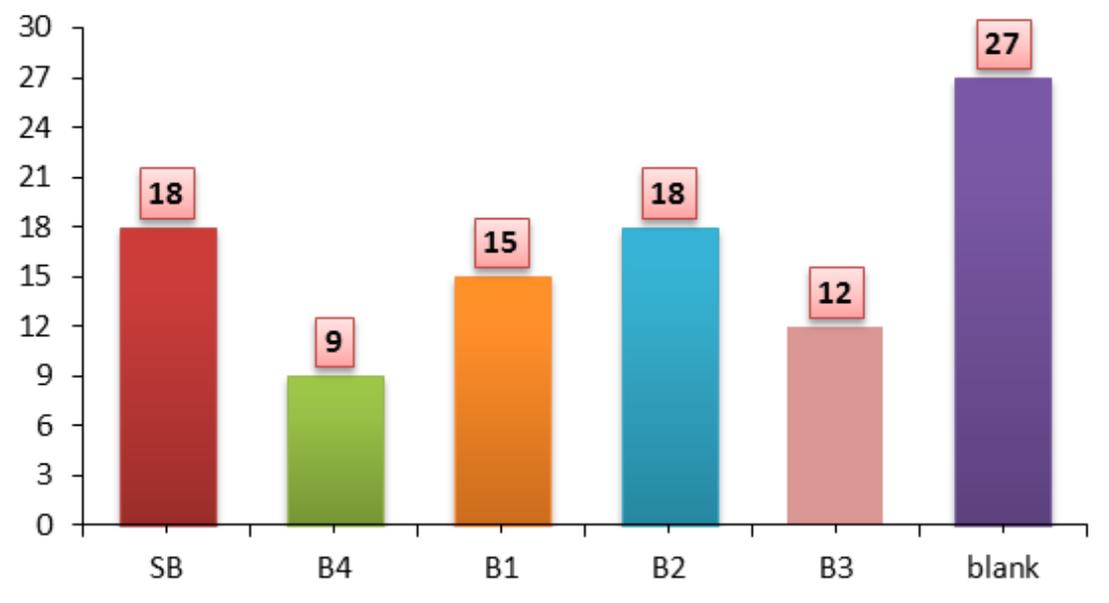
Fig. 8. Pour point degree of [SB1] and its blends at concentration 1000pp
