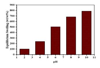
Fig. 2. Swelling performance of the Starch-g-PAAc hydrogel as a function pH.
