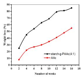
Fig. 6. Biodegradability of the starch-g-PAAc (4:1) hydrogel and AAc over 16 weeks.
