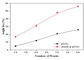
Fig. 7. Biodegradation of the starch-g-PAAc (4:1) hydrogel and AAc over 4 weeks in wastewater model.
