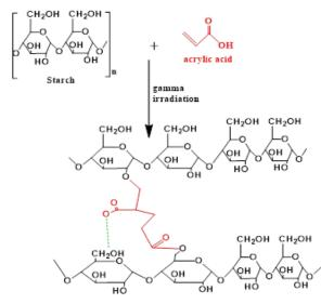
Fig.1. A possible formation reaction of Starch-g-PAAc hydrogel
