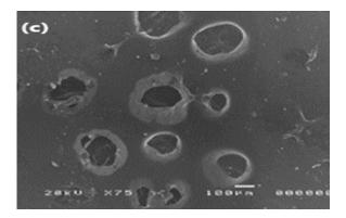
Fig.5. Scanning electron micrograph of Starch-g-PAAc; (a) pH=2, (b) pH=6, (c) and pH=10.
