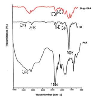
Fig. 3. FTIR spectra of PAAc, Starch, and St-g-PAAc hydrogels.
