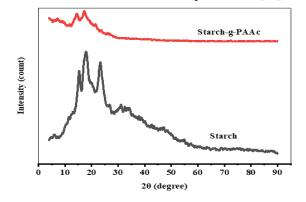
Fig. 4. XRD diffraction patterns of Starch-g-PAAc (4:1) hydrogels.
