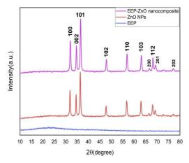
Fig. 1: XRD patterns of EEP, ZnO NPs and EEP-ZnO nanocomposite.
