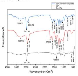
Fig. 3: FT-IR spectrum of ZnO NPs, propolis extract (EEP) and EEP-ZnO nanocomposite.
