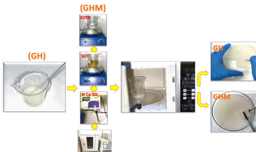
Fig. 1. Schematic preparation of gellan gum (GH) and multi-function gellan gum (GHM) hydrogels.
