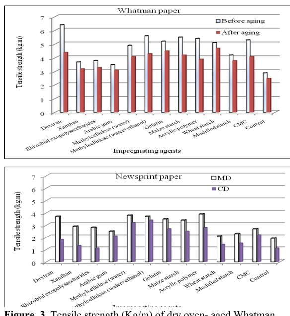
**Figure 3.** Tensile strength (Kg/m) of dry oven- aged Whatman and Newsprint paper treated with different impregnating agents.
