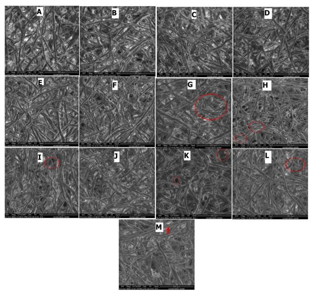
Figure. 5. Study of the surface morphology sheets with scanning electron microscopy (SEM). A: Control, B: Xanthan, C:Dextran, D:Rhizobial polymer, E:Arabic gum, F:Methylcellulose (in water), G: Methylcellulose (in water and alcohol), H: Gelatine, I:Maize starch, J:Acrylic Polymer, K:Wheat starch, L:Modified starch, M:CMC
