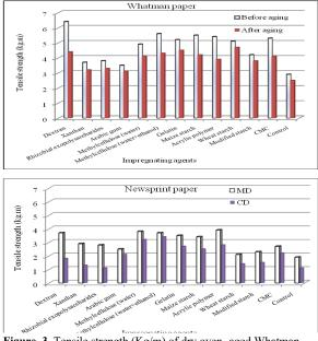
Figure. 3. Tensile strength (Kg/m) of dry oven- aged Whatman and Newsprint paper treated with different impregnating agents. *4.3.2.2. Tearing resistance*
