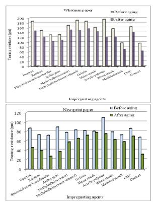
**Figure. 4**. Tearing resistance (gm) of paper treated with impregnating agents before and after aging.
