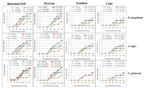
**Figure. 6.** Growth of different fungi on Whatman paper covered with 1.5 % of microbial biopolymer and CMC during 90 days at 25°C in different relative humidity (the growth represented by range of attack).
