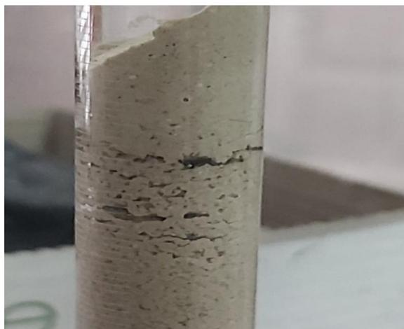
**Figure (7): Percolation leaching upon pelletized sample using glass column**
