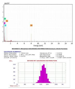
**Figure 14.** Molecular distribution of the synthesized cupper nanoparticles
