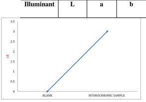
**Figure 3.** Total color differences " $\Delta E$ " between blank and wet hydro-chromic sample–
