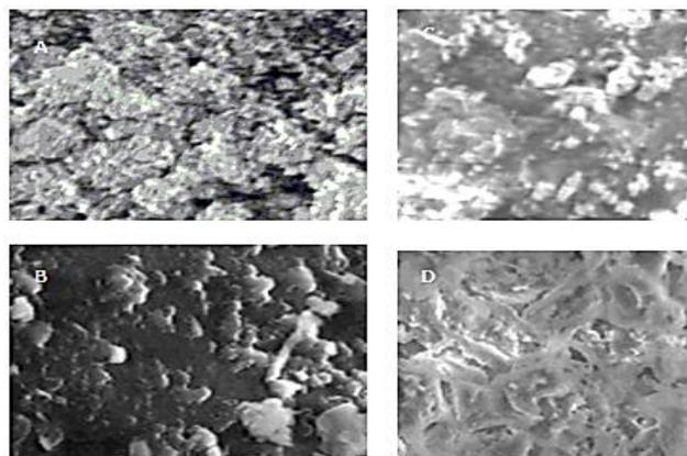
Fig. 10. SEM images of B-8 (a, b), B (c, d) before and after Fe (III), Mn(II) sorption Fe (III), Mn(II) .
