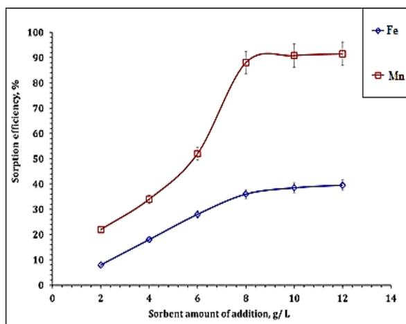
Fig. 6. Effect of adsorbent amount upon Fe (III), Mn(II) adsorption efficiency onto B- 8 (PH 3, 12 h, and room temperature)
