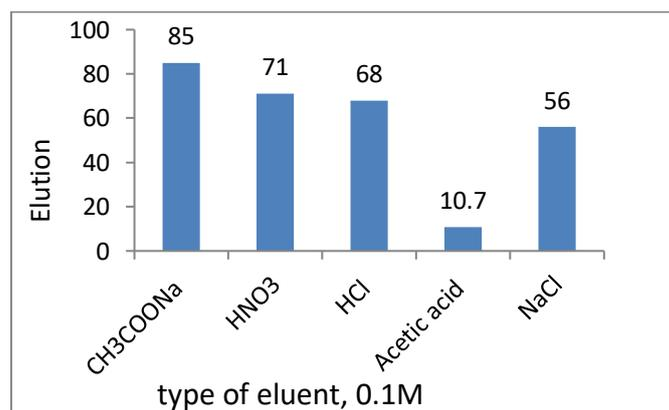
Fig.8: Elution yields using different eluent reagents
