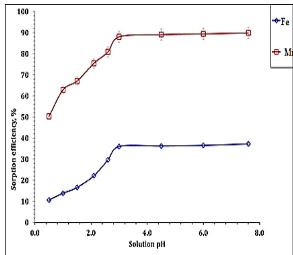
**Fig. 5. Effect of pH upon Fe (III), Mn(II) adsorption efficiency onto B- 8 (0.12 g/15 ml, 12 h and Room temperature)**
