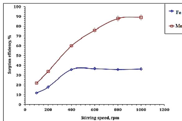
Fig. 7. Influence of agitation moving rpm on Fe (III), Mn(II) sorption effectiveness % (10 h, 0.12 / 15 g/ mL,  $\approx 25^\circ\text{C}$ ).
