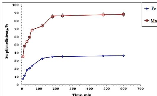
Fig. 1. Influence of the contact time on Fe (III), Mn(II) adsorption efficiency by (B- 8) (0.12 g/15 ml,100 mg/L at ≈ 25 °C and pH 2.9
