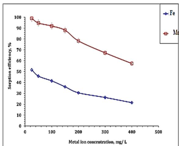
Fig. 2. Effect of initial metal concentration upon Fe (III), Mn(II) adsorption efficiency by (B- 8) (0.12 g/15 ml, 12 h at room temperature and pH 2.9)
