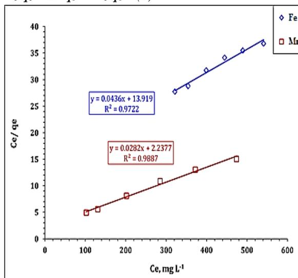
Fig. 3. Langmuir line plans aimed at sorption of Fe (III), Mn(II) onto B- 8.
