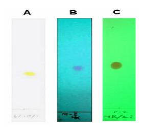
Figure 6: Iodine is used to demonstrate the separation pattern of pure chemicals on a TLC plate (A)., UV light 254 nm (B) and vanillin-sulfuric acid reagent spray (C) for the presence of specific compounds.
