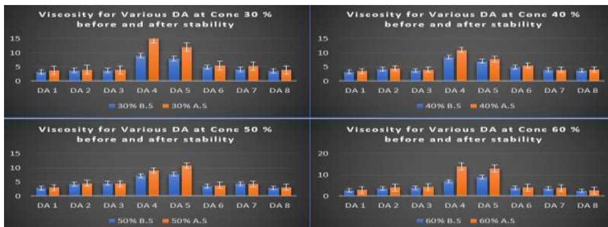
Figure 5 Viscosity for various dispersing agents at different concentrations before and after stability.
