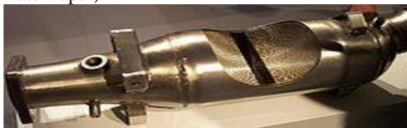
Cross section of a metal-core catalytic converter
