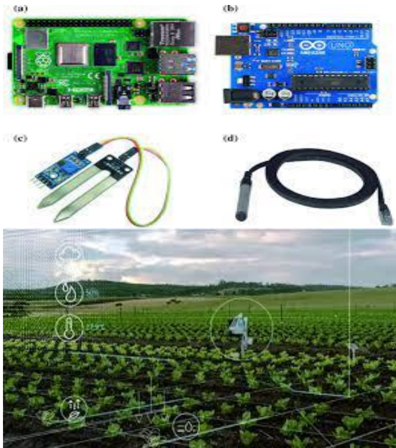
Figure (5): Various devices for smart implementing smart irrigation systems: (a) Raspberry Pi, (b) Arduino, (c) soil moisture sensor, (d) temperature sensor
