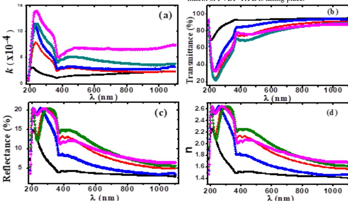
Fig.9: a) The absorption index against  $\lambda$  b) T (%) against  $\lambda$  c) R (%) against  $\lambda$  and d)  $n$  against  $\lambda$ . (■) PVDF-TrFE, (●) 0.5 wt% ZnO/PVDF-TrFE, (▲) 0.75 wt% ZnO/PVDF-TrFE, (▼) 1 wt% ZnO/PVDF-TrFE and (◄) 1.25 wt%
