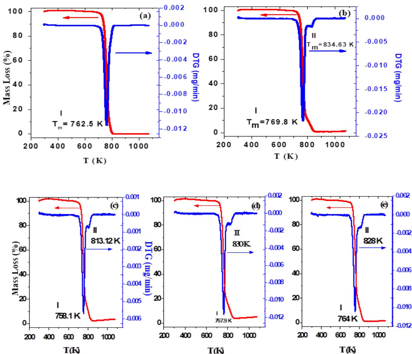
Fig. 4: TGA curve of a) PVDF-TrFE and ZnO/PVDF-TrFE with different concentration of ZnO NPs b) 0.5 wt%, c) 0.75 wt% d) 1 wt% and e) 1.25 wt%.
