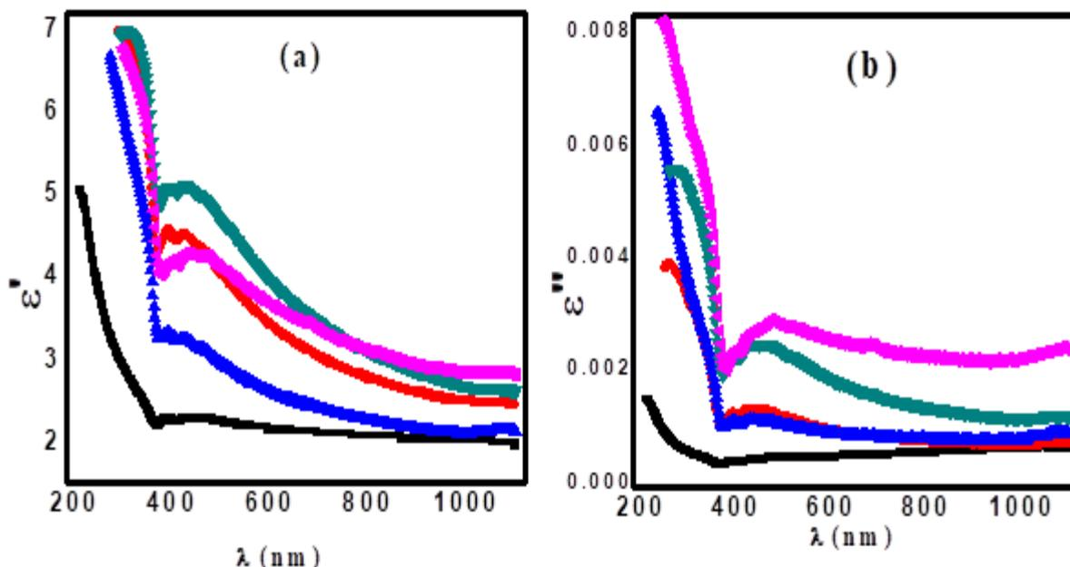
Fig. 11: a)  $\epsilon'$  versus  $\lambda$  and b)  $\epsilon''$  versus  $\lambda$ . (■) PVDF-TrFE, (●) 0.5 wt% ZnO/PVDF-TrFE, (▲) 0.75 wt% ZnO/PVDF-TrFE, (▼) 1 wt% ZnO/PVDF-TrFE and (◄) 1.25 wt% ZnO/PVDF-TrFE.
