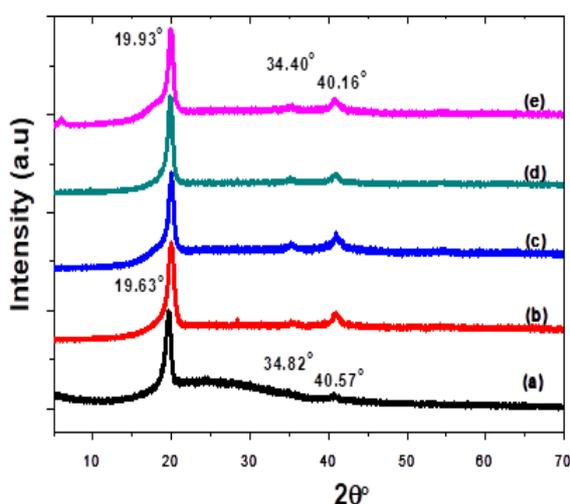
Fig. 1: XRD pattern of a) pure PVDF-TrFE and ZnO/PVDF-TrFE with several contents of ZnONPs b) 0.5 wt%, c) 0.75 wt%, d) 1 wt% and e) 1.25 wt%.
