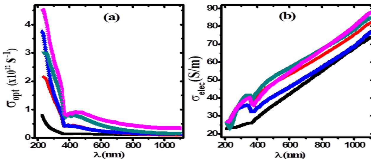
Fig. :12 a)  $\sigma_{opt}$  versus  $\lambda$  and b)  $\sigma_{elec}$  versus  $\lambda$ . (■) PVDF-TrFE, (●) 0.5 wt% ZnO/PVDF-TrFE, (▲) 0.75 wt% ZnO/PVDF-TrFE, (▼) 1 wt% ZnO/PVDF-TrFE and (◀) 1.25 wt% ZnO/PVDF-TrFE.
