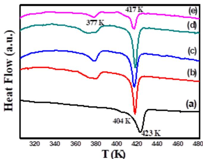
Fig. 3: DSC of a) PVDF-TrFE and ZnO/PVDF-TrFE with different concentration of ZnO NPs b) 0.5 wt%, c) 0.75 wt%, d) 1 wt% and e) 1.25 wt%.
