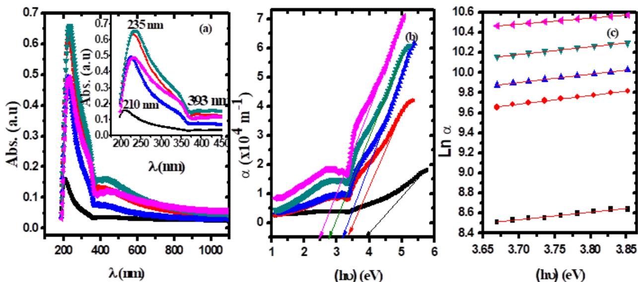
Fig. 7: a) The absorption versus  $\lambda$  b)  $\alpha$  versus  $h\nu$  and c)  $\ln \alpha$  versus  $h\nu$ . (■) PVDF-TrFE, (●) 0.5 wt% ZnO/PVDF-TrFE, (▲) 0.75 wt% ZnO/PVDF-TrFE, (▼) 1 wt% ZnO/PVDF-TrFE and (◄) 1.25 wt% ZnO/PVDF-TrFE.
