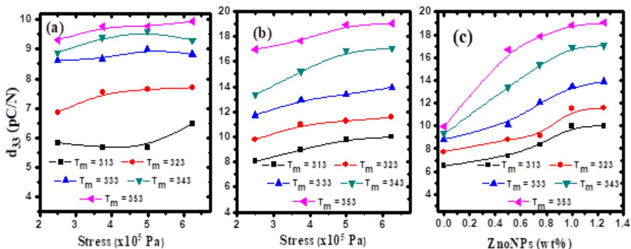
Fig. 13: The piezoelectric coefficient ( $d_{33}$ ) against the stress at different measuring temperatures for a) pure PVDF-TrFE b) 1.25 wt% ZnO/PVDF-TrFE and c)  $d_{33}$  versus ZnO NPs ratio. The samples are poled with  $E_p=1 \times 10^7$  V/m at  $T_p=353$  K for  $t_p=20$  min and the applied stress is  $6.24 \times 10^5$  Pa.
