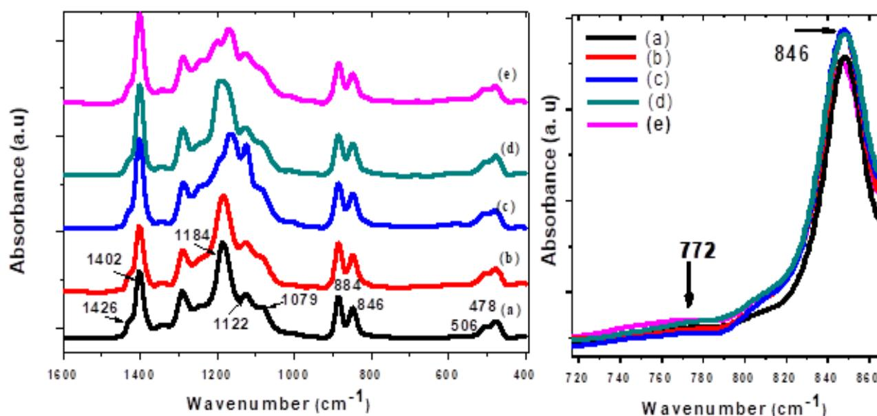
Fig. 2: FTIR spectra of a) pure PVDF-TrFE and ZnO/PVDF-TrFE with different concentrations of ZnONPs b) 0.5 wt%, c) 0.75 wt%, d) 1 wt% and e) 1.25 wt%.
