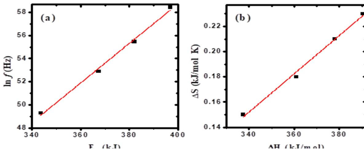
Fig. 6: a)  $\ln f$  versus  $E_a$  and b)  $\Delta S$  versus  $\Delta H$  in the first stage.
