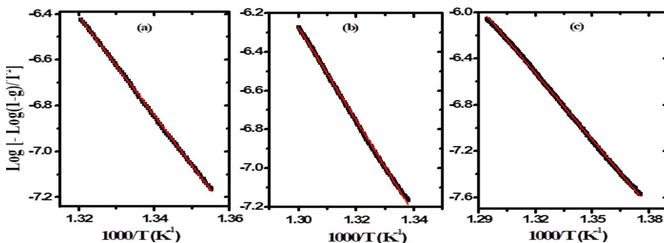
Fig. 5: Log  $[-\log(1-g)/T^2]$  versus  $1/T$  for a) pure PVDF-TrFE, b) 0.5 wt% ZnO/PVDF-TrFE and c) 1 wt% ZnO/PVDF-TrFE NCs.
