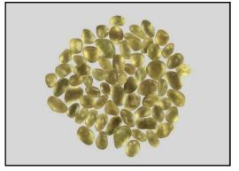
Fig. 11. High-grade monazite concentrate resulted from the concentration processes of the black sands.
