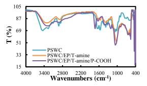
Fig. 1. FTIR spectra of PSWC, PSWC/EP/T-amine and PSWC/EP/T-amine/P-COOH adsorbents
