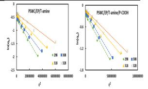
Fig. 9. The Dubinin-Radushkevich isotherm for lanthanum adsorption by PSWC/EP/T-amine and PSWC/EP/T-amine/P-COOH
