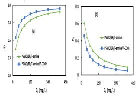
Fig. 8. The monolayer surface coverage (a) and separation factor (b) for lanthanum adsorption by PSWC/EP/T-amine and PSWC/EP/T-amine/P-COOH.
