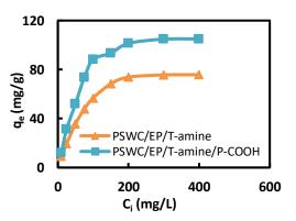
Fig. 5. The effect of adsorbate concentration on lanthanum adsorption by PSWC/EP/T-amine and PSWC/EP/T-amine/P-COOH
