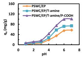
Fig. 3. Effect of solution pH on uptake of lanthanum ions PSWC/EP, PSWC/EP/T-amine, and PSWC/EP/T-amine/P-COOH
