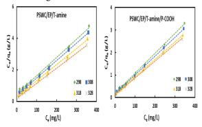
Fig. 7. Langmuir isotherm of lanthanum adsorption by PSWC/EP/T-amine and PSWC/EP/T-amine/P-COOH.
