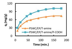
Fig. 4. Effect of time on lanthanum adsorption by PSWC/EP/T-amine and PSWC/EP/T-amine/P-COOH.
