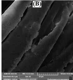
**Fig. 6.** SEM images of untreated fabric (A) and PDMS emulsion (40 g/L) treated fabric (B).
