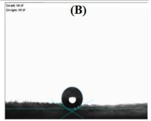
Fig. 8. Images of water droplets on surface of the water repellent fabric samples treated with the PDMS emulsion (40 g/L) and then dried at 100  $^{\circ}$ C (A) or 160  $^{\circ}$ C (B).
