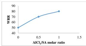
**Fig. 2.** Effect of AlCl<sub>3</sub>/SA molar ratio on WRR of treated fabric. The PDMS emulsion ingredients: PDMS (5%); SA (4.5%) and TEA (2.4%). The fabric is treated with 50 g/L of mother emulsion and then dried at 100  $^{\rm O}$ C/5min.
