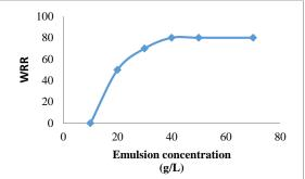
Fig. 3. Effect of emulsion concentration on WRR of treated fabric. The PDMS emulsion ingredients: PDMS (5%); TEA (2.4%); SA (4.5%); and AlCl<sub>3</sub>/SA molar ratio 1. The fabric is treated with different emulsion concentrations and then dried at  $100 \text{ }^{\circ}\text{C/5min}$ .
