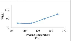
**Fig. 4.** Effect of drying temperature on WRR of treated fabric. The PDMS emulsion ingredients: PDMS (5%); SA (4.5%); TEA (2.4%) and AlCl<sub>3</sub>/SA molar ratio (1/1). The
