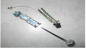
Figure 7: Nickel cannon cathodes from TVs
