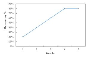
Figure 5: Effect of fusion time on lead recovery at 1100 °C as fusion temperature.
