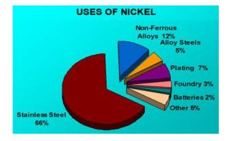
Figure 13: uses of Nickel
