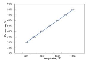
Figure 4: Effect of iusion temperature on lead recovery for 2 hr as fusion time.
