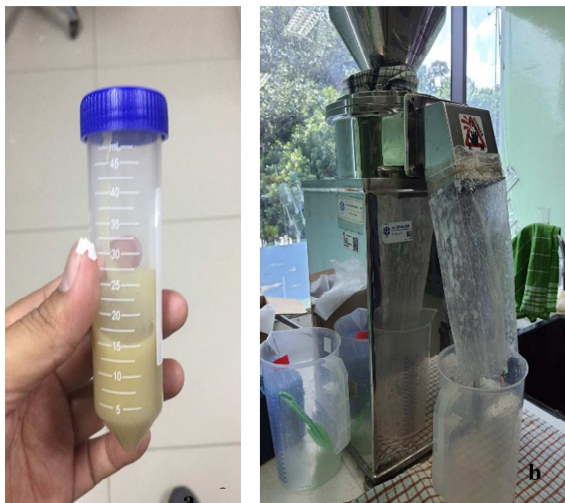
Fig. 2: CNC results (a) from cellulose disintegrations of ultrafine grinding machine (b)
