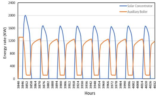
**Figure 12:** Energy rate delivered from Collector and Auxiliary Boiler from 10-17 June
