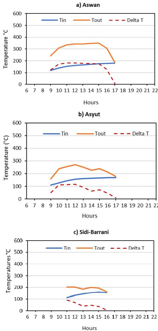
**Figure 10:** The inlet, outlet, and temperature raised of HTF through the solar concentrator on a day in Winter (15 January) for a) Aswan b) Asyut c) Sidi-Barani
