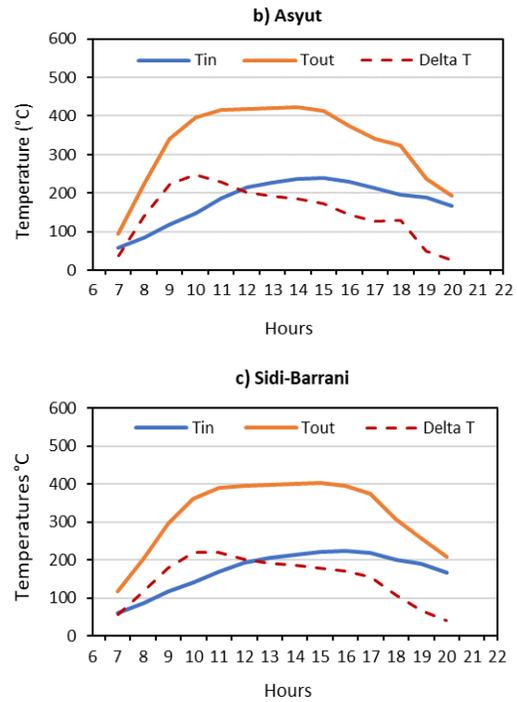
**Figure 11:** The inlet, outlet, and temperature raised of HTF through the solar concentrator on a day in Summer (15 June) for a) Aswan b) Asyut c) Sidi-Barani
