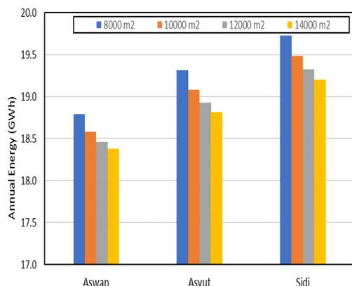
**Figure 15:** The annual energy required by the boiler at the three selected Sites with different PTC aperture areas
