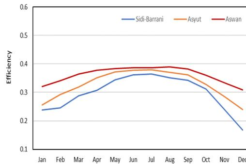
Figure 9: Solar field efficiency for the three select regions through one year
