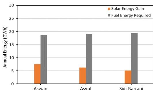
**Figure 14:** The Collector Energy Gained and Boiler Energy Required Annually for the Selected Sites
