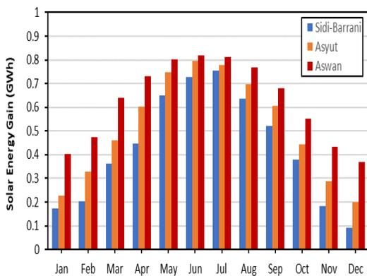
Figure 7: Energy gained from the solar field each month
