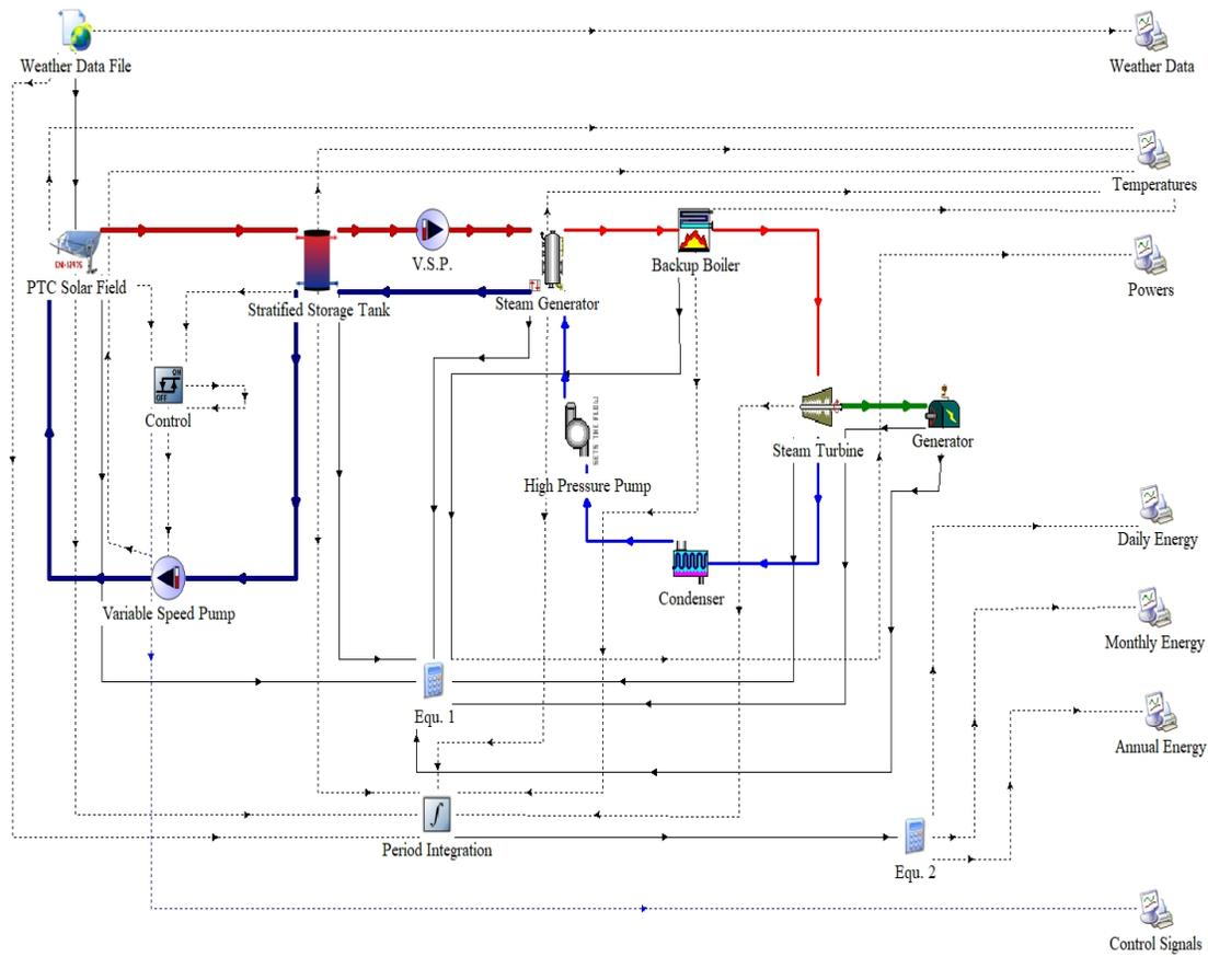
Figure 3: TRNSYS simulation model of the plant
