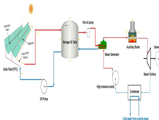
Figure 1: Schematic diagram of the solar thermal power plant
