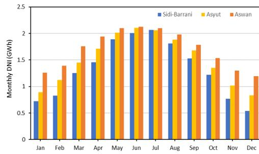
Figure 8: Monthly DNI gained from the solar field
