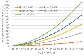
Fig. 7: Effect of plate diameter (surface area) on the hydrogen production rate for different number of cells
