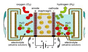
Fig. 3: Schematic diagram of operation of an alkaline electrolysis cell
