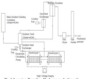
Fig. 4: Layout configuration of hydrogen production unit
