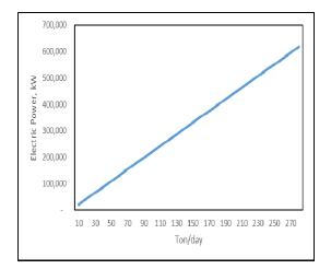
Fig. 9: The required electric power as a function of the amount of H<sub>2</sub> production in ton/day
