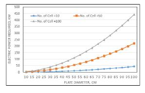
Fig. 8: Effect of plate surface area on the electric power required, kW for different number of cells
