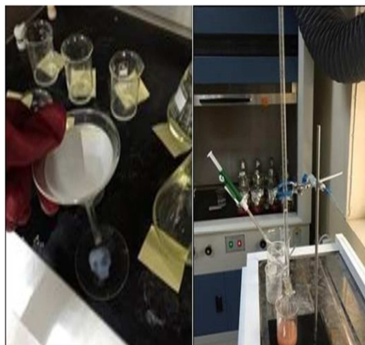
Figure 1: Determination the main composition of Cement
