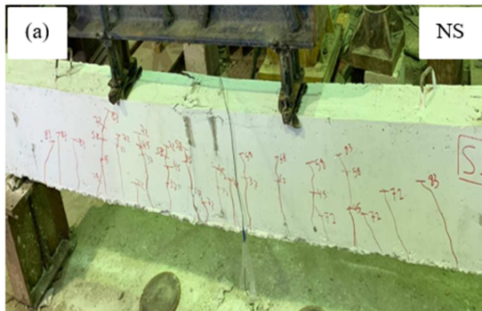
Figure 14: Crack patterns and failure shapes of normal concrete with steel reinforcement
