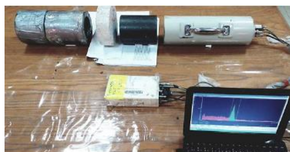
a) Attenuation coefficient experimental setup
