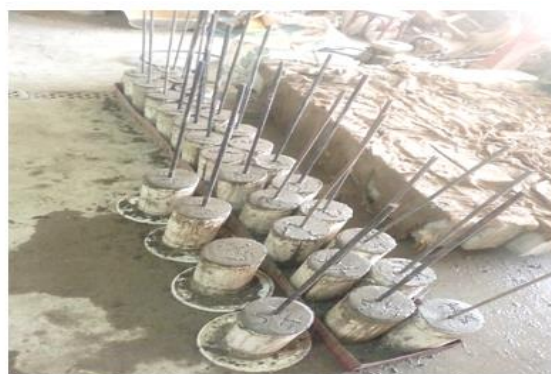
a) Pull-out test specimens' preparation
