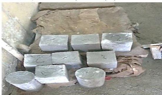
b) Part of standard cubes and cylinders after curing
