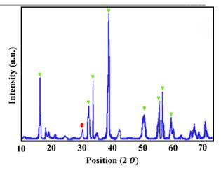
Fig. 3 XRD pattern of prepared sodium zirconate.
