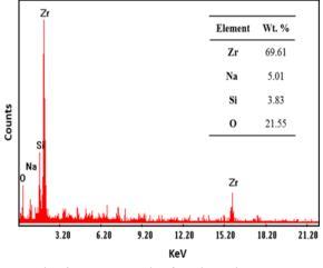
Fig. 4 EDX analysis of sodium zirconate.
