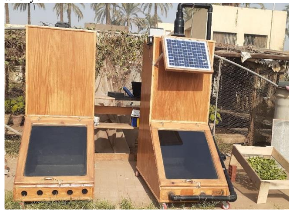
Fig.3 Front view photo for the three dryers (UMISD, MISD and DSD)
