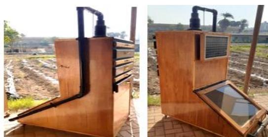
Fig.2. (A). The side view photo of the MISD solar dryer.
