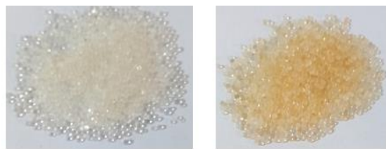
Fig.13. Silica gel before drying at 8 a.m.(A), Silica gel after drying at 3 p.m. (B).
