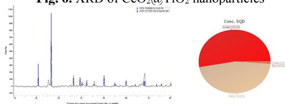
Fig. 6. XRD of \text{CeO}_2@\text{TiO}_2 nanoparticles
