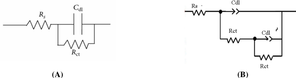
Fig. 21. Electrochemical equivalent circuit model used for EIS data fitting (A) for Bare electrode, (B) for SS coated with M- POM/ CoFe 2 O 4 -SiO 2 epoxy.
