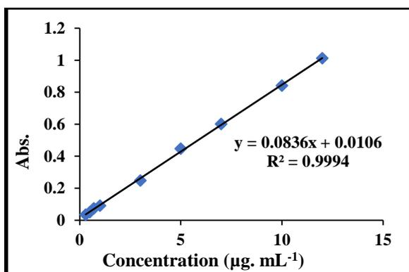
**Figure 4.** Calibration curve of nitrite ion determination.
