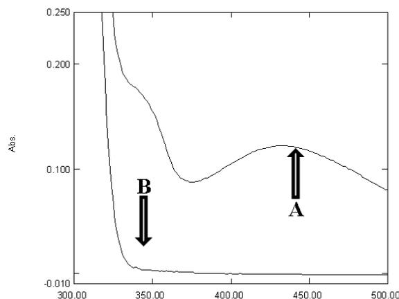
**Figure 2.** Absorption spectra of (A) azo dye of nitrite ion against blank (B) blank against D.W.
