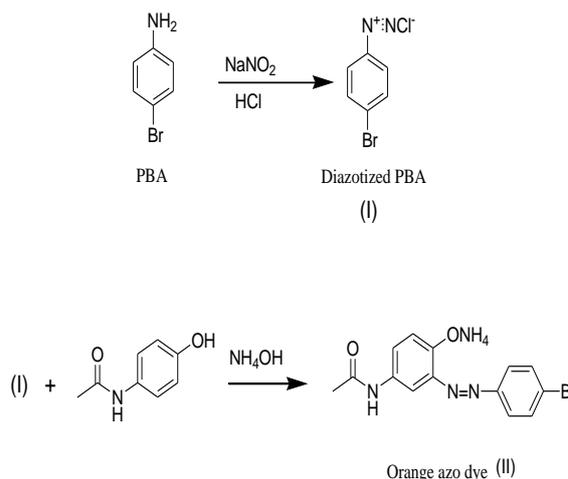
**Scheme 1: Schematic diagram of azo-dye formation.**
