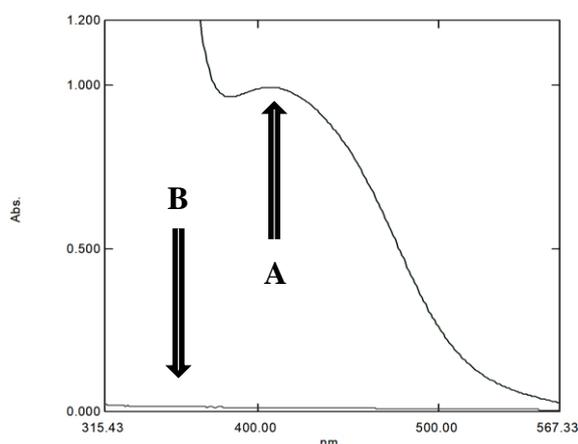
**Figure 5.** Absorption spectrum of (A) Extracted azo dye against reagent blank, and (B) blank against solvent.
