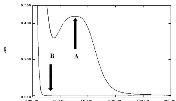
**Figure 3.** Absorption spectrum of (A) azo dye against reagent blank (B) blank against distilled water.
