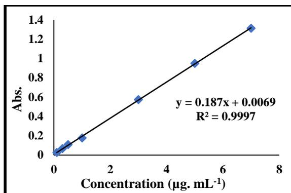
**Figure 7.** Calibration graph of Nitrite ion determination by DLLME method.**Table 6.** The statistical data of the calibration curve obtained using DLLME-spectrophotometric determination of nitrite ion.
