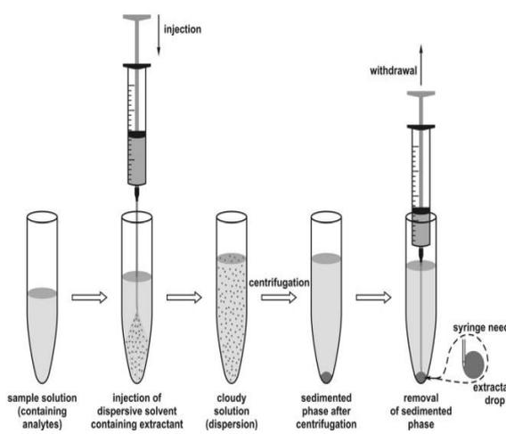
**Figure 1. Mechanism of DLLME [26].**
