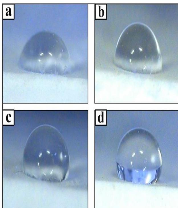
Fig. 5. The results of measuring the water contact angle of untreated glazed pottery samples and treated/consolidated samples.
