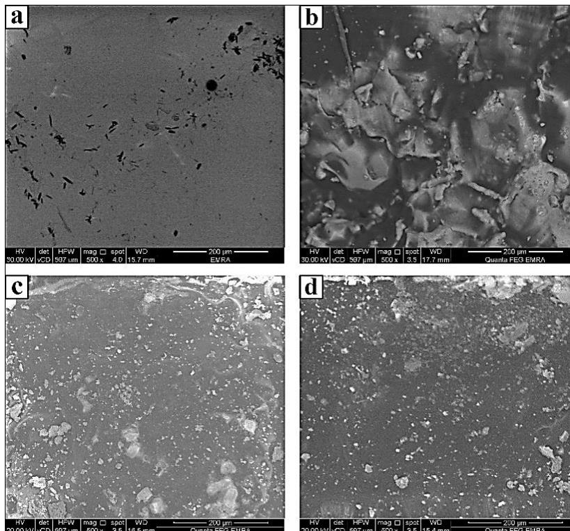
**Fig. 4.** SEM microscope images of the untreated and treated/consolidated samples. (a) Untreated sample, (b) the sample treated/consolidated with Wacker OH100, (c) sample treated/consolidated with Wacker OH100 + Nano Silver 1% nanocomposite, (d) the sample treated with Wacker OH100 + Nano Silver 3% nanocomposite.
