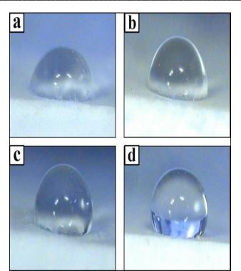
Fig. 5. The results of measuring the water contact angle of untreated glazed pottery samples and treated/consolidated samples.
