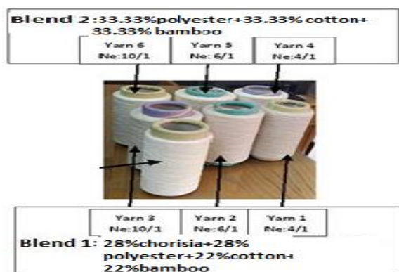
Fig. 2. produced weft yarns at different counts and fiber formulations
