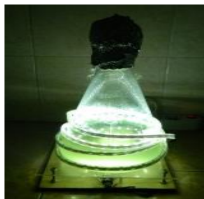
Fig. 3. Irradiation of algae using white LEDs source for twenty-one days.
