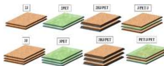
Figure 1. Schematic diagram of the laminated composite samples layers' structure prepared from jute and polyester nonwovens.
