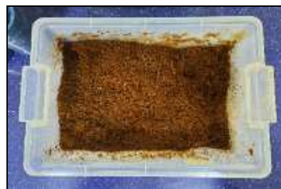
Figure 2. The compost reactor box.
