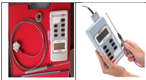
Figure 2.2.3GM07 Gauss meter with Transverse probe
