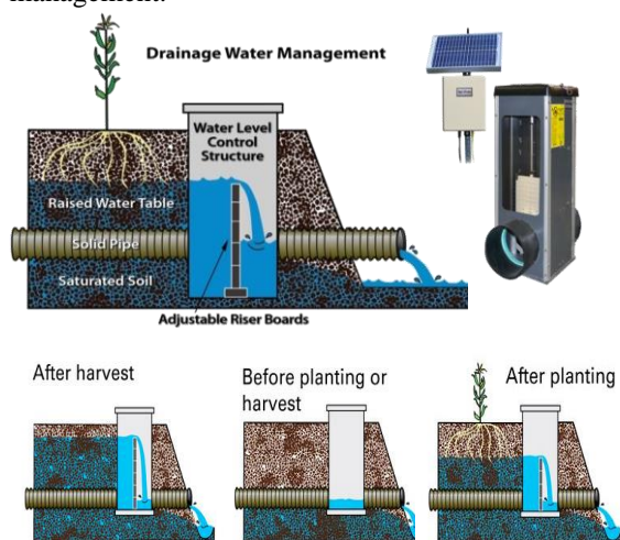
Fig. 9. Riser board for drainage water management.
