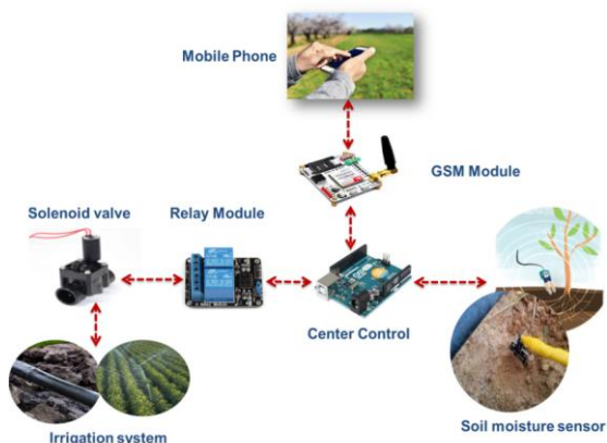
Fig. 7. The components of automatic irrigation with an ARDUINO system.
