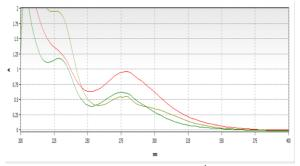
Fig. 2. Absorbance spectra of AMT 20  $\mu$ g ml<sup>-1</sup> (I), MET 20  $\mu$ g ml<sup>-1</sup> (II) and PPZS(III) 20  $\mu$ g ml<sup>-1</sup> in 0.1N HCl.
