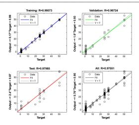
Fig. 4. Predicted concentration plots vs. real concentration for tertiary mixture by ANN ( $\mu g \ ml^{-1}$ ).
