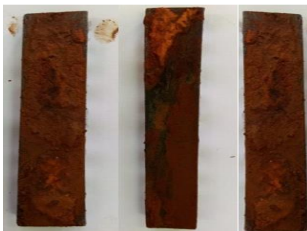
Fig. 6: Shows the iron coupons during corrosion in bottles and the coupons after the test
