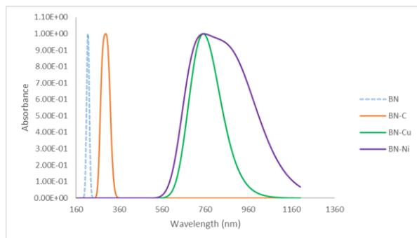
**Figure 4: The UV-Visible spectrum of pure and doped BN nano systems computed by TD-DFT at basis set LAN2DZ with hybrid function B3LYP**
