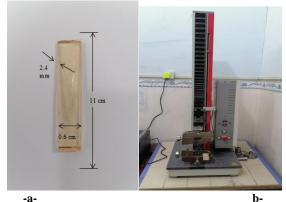
Fig 1: a-shows the tensile strength test sample.b-Shows mechanical properties measuring device (Tensile).
