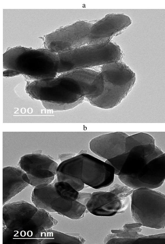
Fig. 3 TEM of a) diatomite and b) Cu-MOF/diatomite
