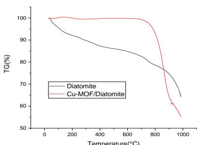
Fig. 4 TGA of diatomite and Cu-MOF/diatomite.
