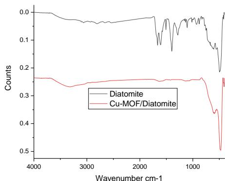
Fig. 1 FTIR of diatomite and Cu-MOF/diatomite
