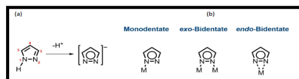
Figure (1). (a) Deprotonation of 1H-pyrazole to produce pyrazolate, (b) Coordination modes of pyrazolate to a metal, in organometallic chemistry.
