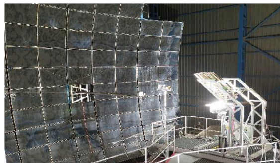
Fig. 1. Aspect of the parabolic concentrator and the test platform (with mirror reflector inclined at 45 degrees) of the oven SF60 of the Solar Platform of Almeria.
