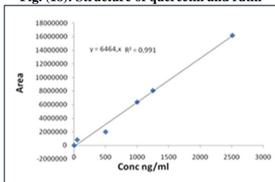
**Fig. (19): Calibration curve of rutin**
