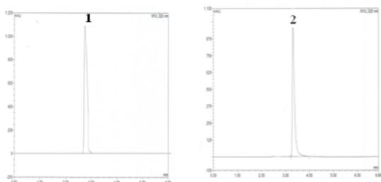
**Fig. (10): HPLC chromatogram of cinnamic acid standard**
