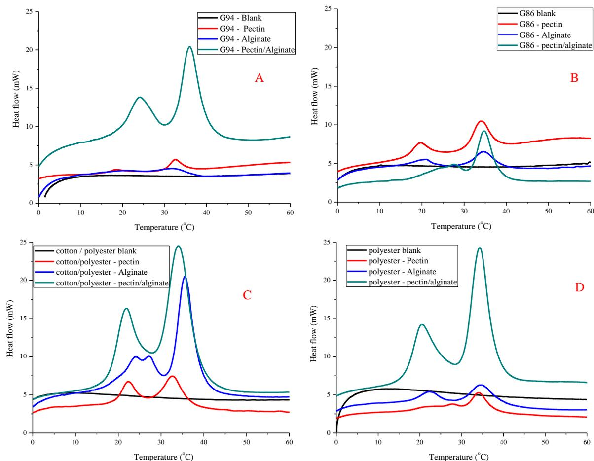
Figure 3: DSC curves for covered yarns with pectin or alginate/stearic acid and Octadecane at 2<sup>nd</sup> heating
