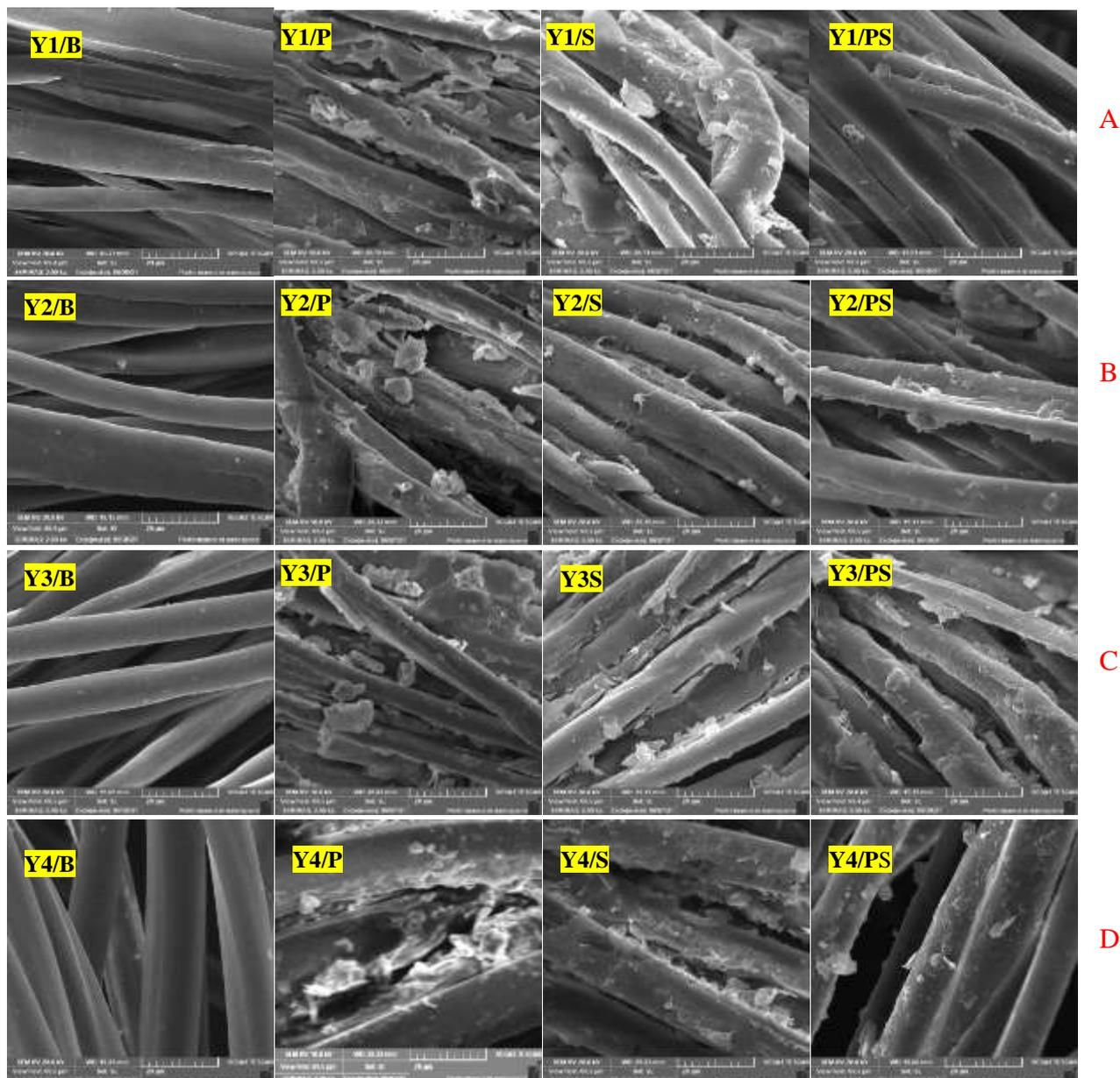
Figure 4: SEM of different yarn materials after applying PCMs treatments
