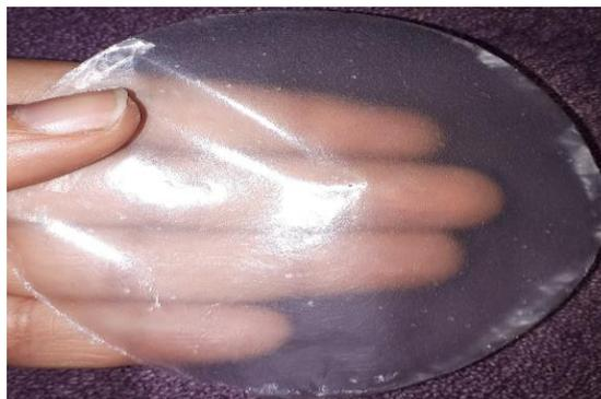
Fig 9 Nanochitosan membrane
