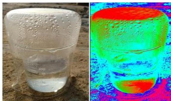
Figure 3: Water evaporation of saline water, and the corresponding thermal picture
