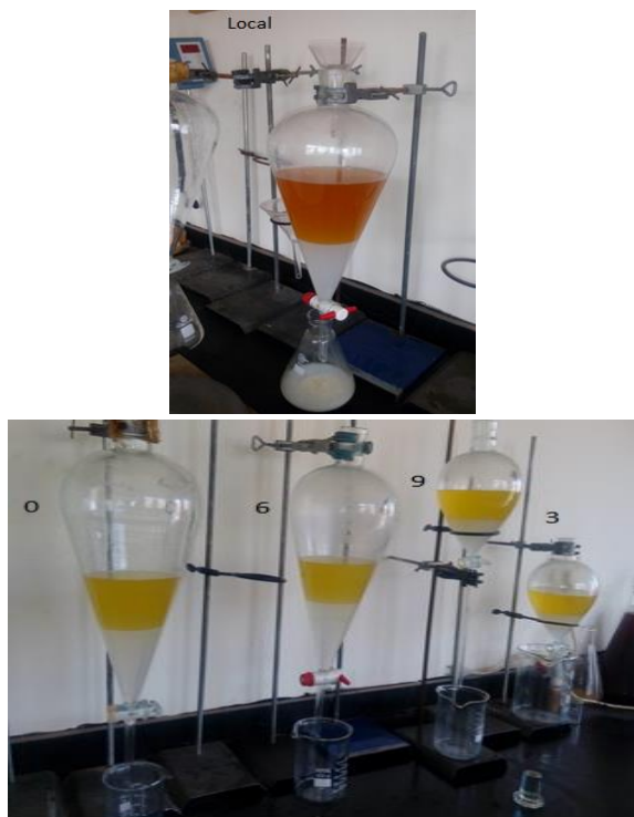
Fig. 6 Washing and Drying of Biodiesel.
