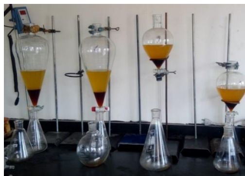
Fig. 5 Settling and Separation of Biodiesel.
