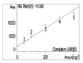
**Figure 3**: Calibration curve for Thiamethoxam (concentration from 50-400 mg/L).
