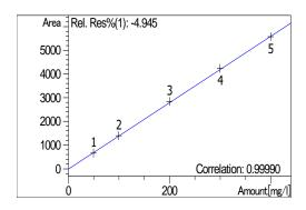
**Figure 2**: Calibration curve for Spirodiclofen (concentration from 50-400 mg/L).(concentration from 50-400 mg/L).
