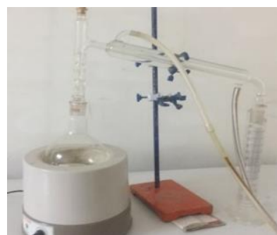
Figure 4. Separation EG from DPET process.
