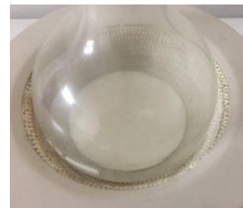
Figure 3. The PET and EG became one homogenous mixture, frizzed at RT.
