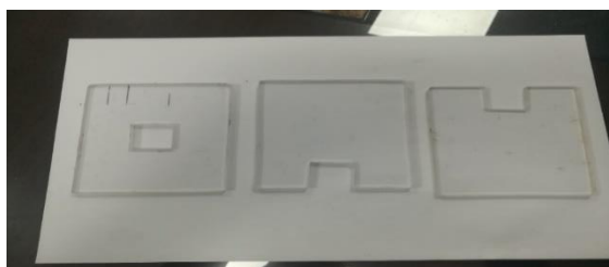
Figure.5. The Shapes of partions are put in Perspex Channel to create waving in an open channel.
