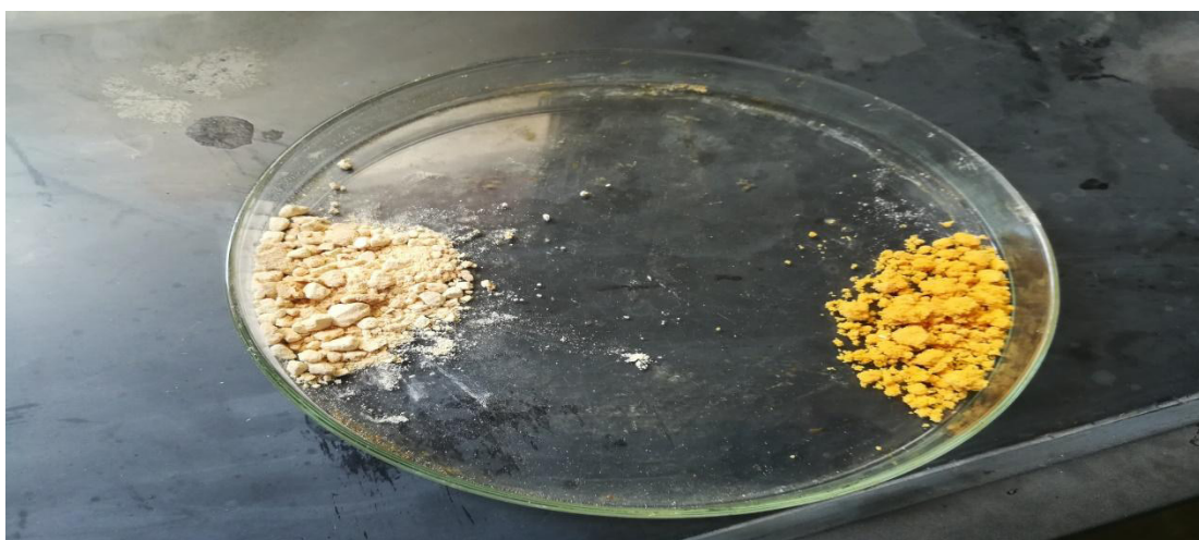
Fig. 18. Left side shows the fresh micro-capsules while the right side shows the micro-capsules after four months One shell micro-capsules
